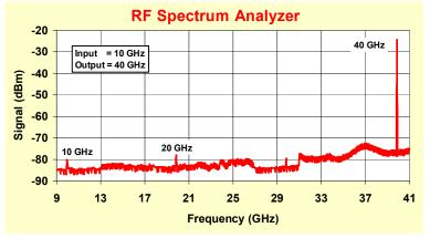
The Equalizer micrometer adjusts the amplitude of one pulse leg so that the two recombined pulses have equal amplitude. The suppression of the input frequency is at least 35 dB.
